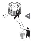
Check if the surface of the cartridge is torn; in this case, the filter cartridge cannot be used any longer.
